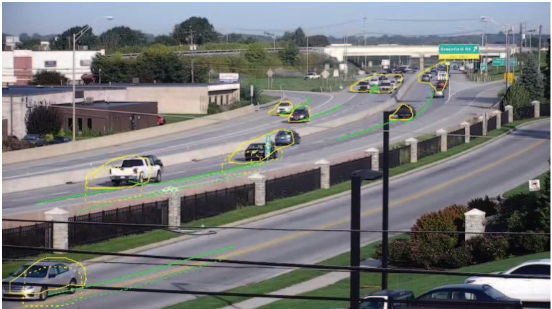
Image from visible imager with VCA metadata and trajectory lines
