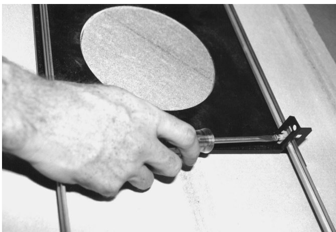
Figure 9.3: Tighten Bracket Securing Screw
